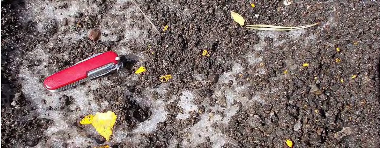
Yellow paint chips mixed with gravel on snow near Rainbow Bridge (DSCN6021.JPG).
